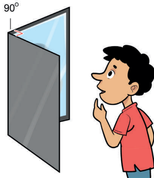
Image: The reflection in two mirrors placed at right angles does not invert right-left.
